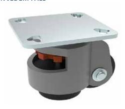
The fixing takes place with a bolt hole thread using double-threaded bolts in transport and base plates or core holes of aluminum profiles. The leveling castors can also be ordered with a mounting plate for flush mounting on modular dimension 40 and 45.
